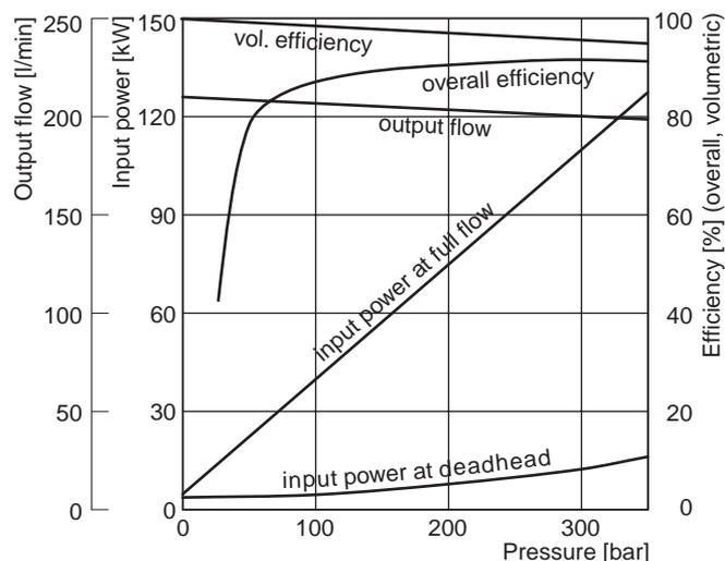
**Efficiency and case drain flows PV140, PV180, PV270**
