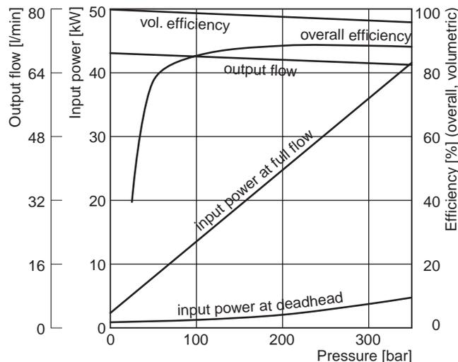
**Efficiency and case drain flows PV032, PV040, PV046**
