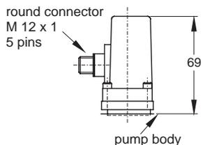
**Pilot valve for horse power compensator**
