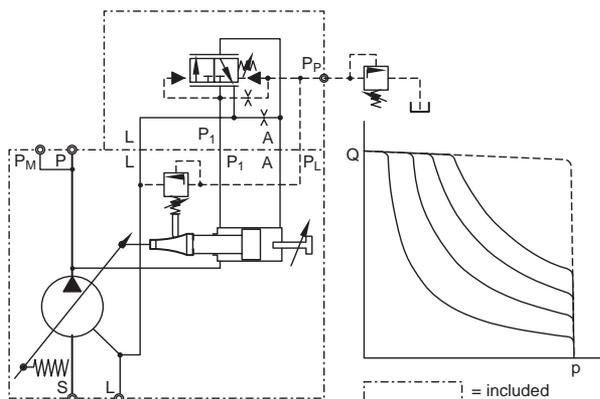
**Pump with Electrohydr. Displacement Control, code FPV**
