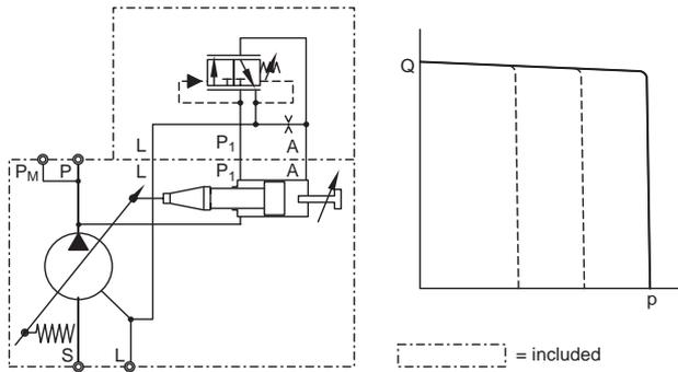
**Pump with Load-Sensing Compensator, code FFC**
