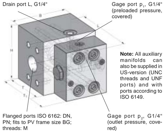
**Note:** All auxiliary manifolds can also be supplied in US-version (UNC threads and UNF ports) and with ports according to ISO 6149.
