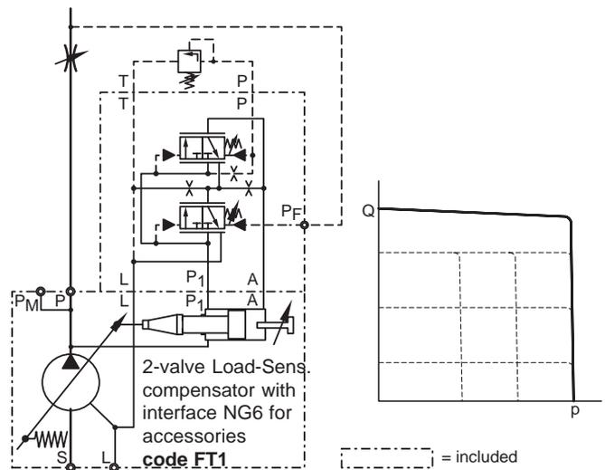
**Hydraulic-mechanical horse power compensator**
