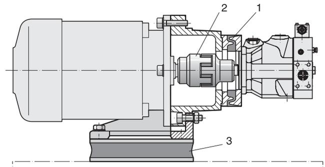
1) Bell housing                      2) Coupling                      3) Damping rails
