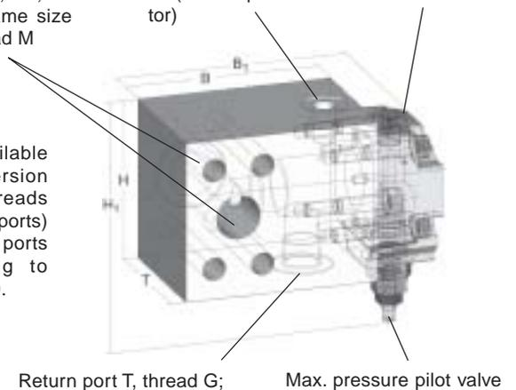
**Dimensions quick unload manifold PVAPSE\***
