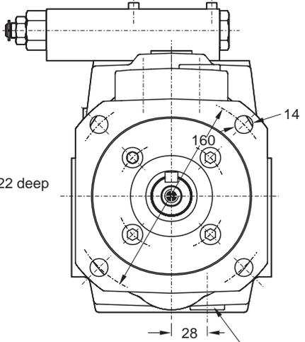
flushing port L3; G 1/2 optional M 22 x 1.5; ISO 6149-1 (threads options 7 and 8) oder 7/8 - 14 UNF (threads option 3)
