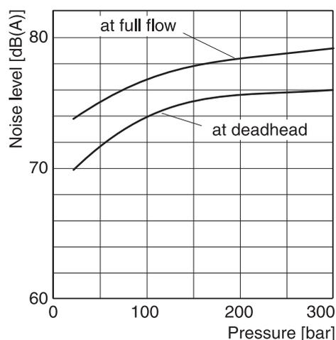
Typical sound level for single pumps, measured in anechoic chamber according to DIN 45 635, part 1 and 26. Microphone distance 1m; speed:  $n = 1500 \text{ min}^{-1}$ .
