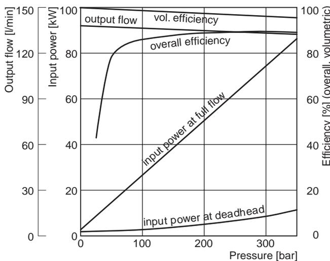
**Efficiency and case drain flows PV063, PV080, PV092**
