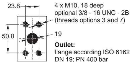
The pump shown above has **mounting option K**
