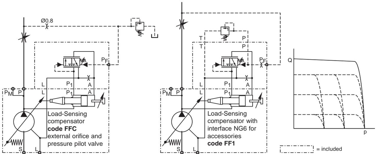
Shown above is **load-sensing compensator, code FF1** with an NG6 interface on top of the control valve. That allows direct mounting of a pilot valve for pressure compensation. This version includes the pilot orifice.
