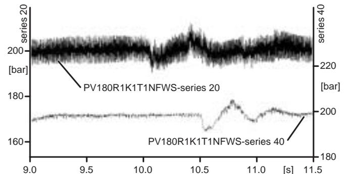
**Figure 2:** Comparison of the pressure pulsation in a system with 6 old PV pumps versus the same system with 6 PVplus pumps. The pulsation reduction effect of the precompression volume is evident.
