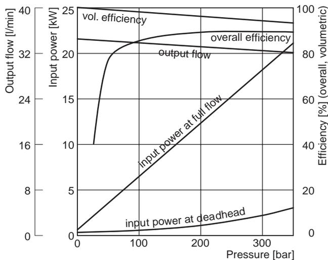
Efficiency and case drain flows PV016, PV020, PV023
