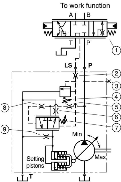
1. Directional, load sensing control valve
