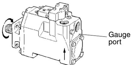
Fig. 4. Left hand rotating pump.
