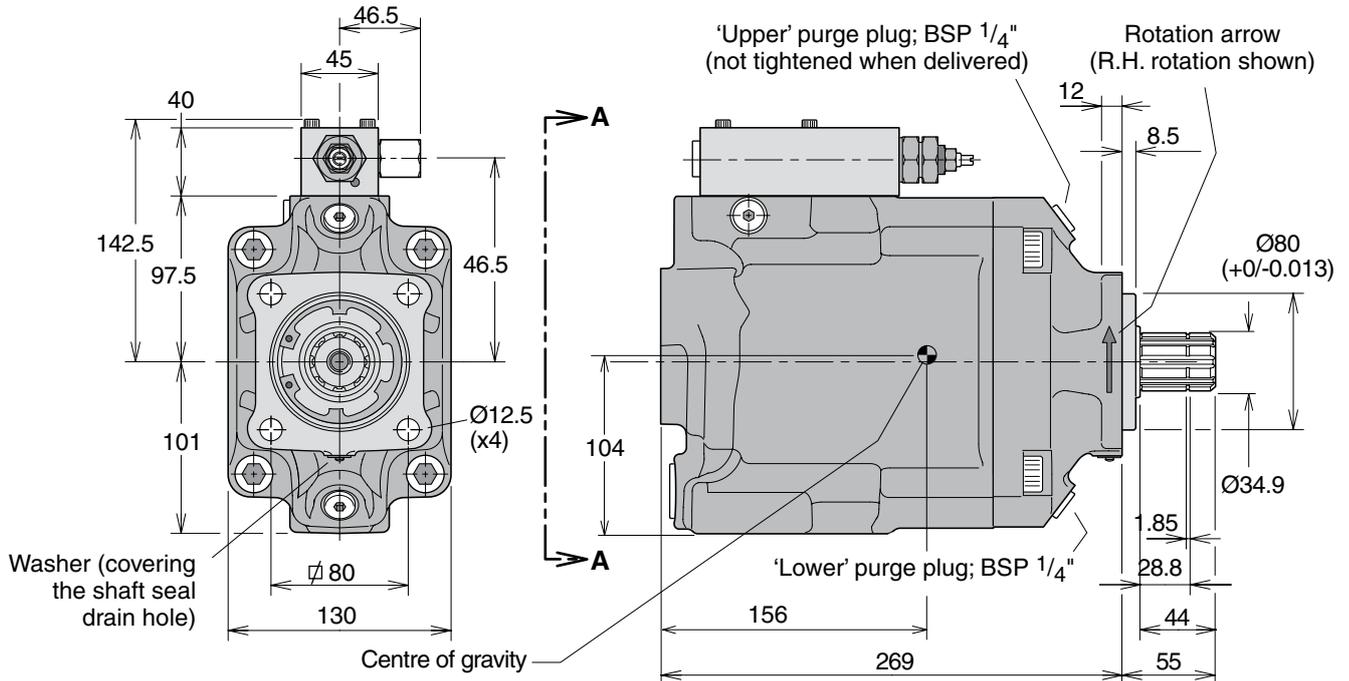
**NOTE:** The pump **does not** include a suction fitting; it must be ordered separately. See chapter 10-3.
