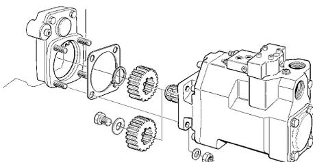
Fig. 6. VP1-to-PTO installation.
