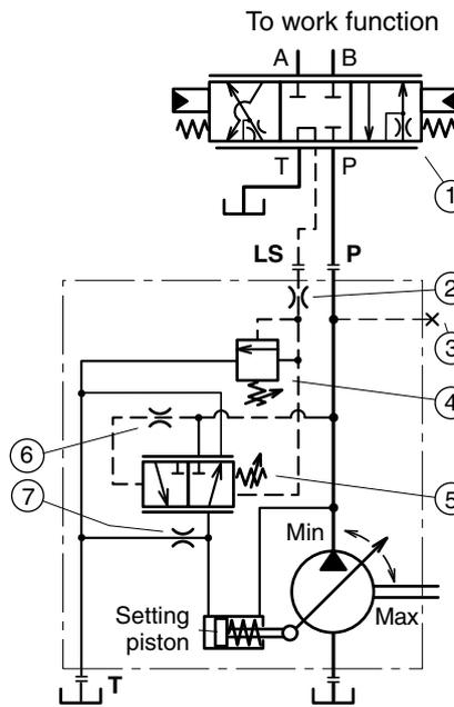
1. Directional, load sensing control valve
