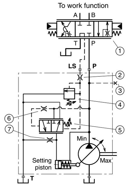
1. Directional, load sensing control valve
