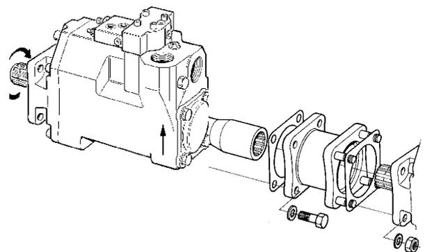
Fig. 3. Adaptor kit (P/N 379 7795) for tandem coupling.
