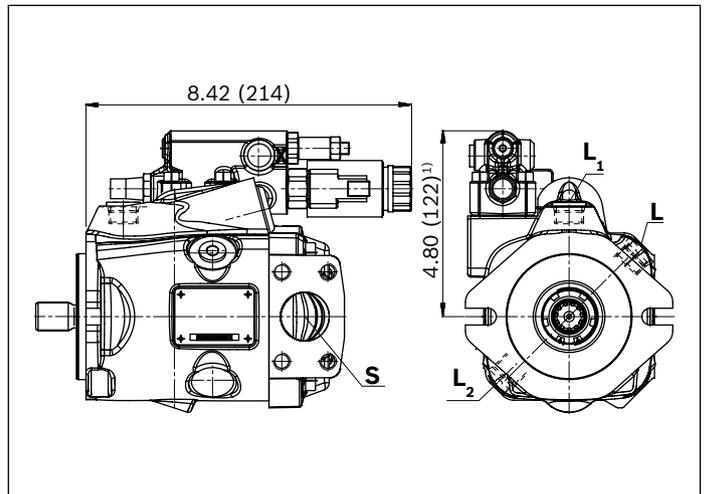
1) ER7.: 6.18 inch (157 mm) if using an intermediate plate pressure controller
