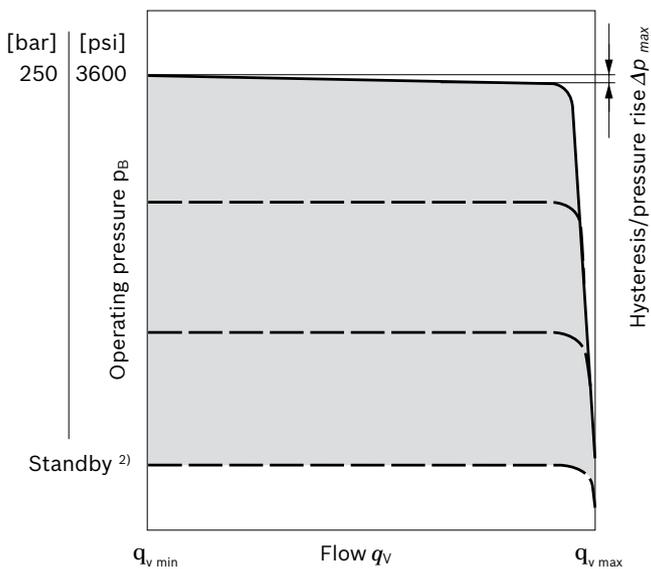
Characteristic curve valid for  $n_1 = 1500$  rpm and  $t_{\text{fluid}} = 120$  °F (50 °C).
