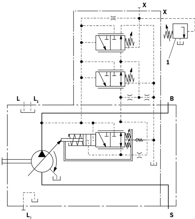
**1** The sensing orifice (control block) and the line is not included in the delivery contents.
