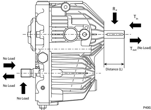
The maximum shaft thrust in ( $T_{in}$ ) of input shaft is 18% of allowable radial load ( $R_e$ ) of the input shaft. The shaft thrust out ( $T_{out}$ ) of the input shaft should be no load. The radial and thrust load of the output shaft should be no load.
