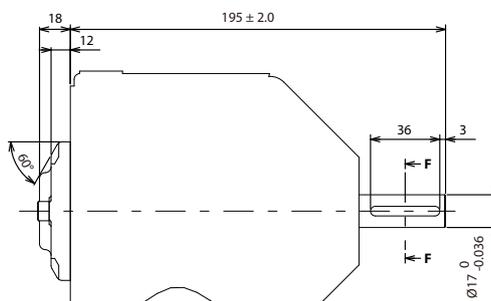
Pump Shaft : 17mm Straight Keyed (Key Length 36mm)
