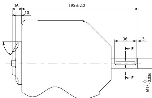
Pump Shaft : 17mm Straight Keyed (Key Length 36mm)
