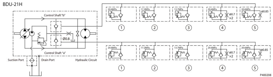
1. Check Valve with Relief Valve, Option Code.: R0
