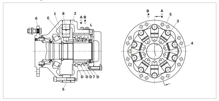
Hydraulic motors of the type MCR-C are radial piston motors with rear case mounting and flanged drive shaft. These motors have a compact front housing and are intended for drives in open or closed circuits. These motors are used in a wide range of applications where there is lower external loading. The integrated flange with wheel studs allows easy installation of standard wheel rims.
